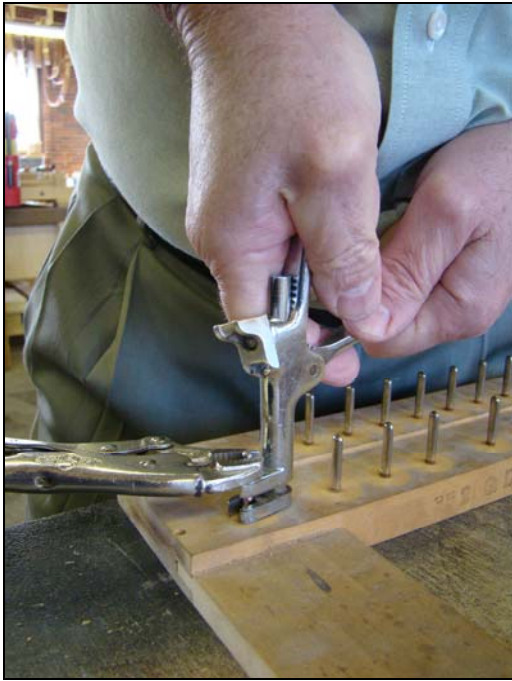
Figure 6 Removing front rail pins with vice grips and puller
