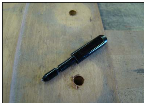
Figure 8 New Front Rail Pin with oversize hole
