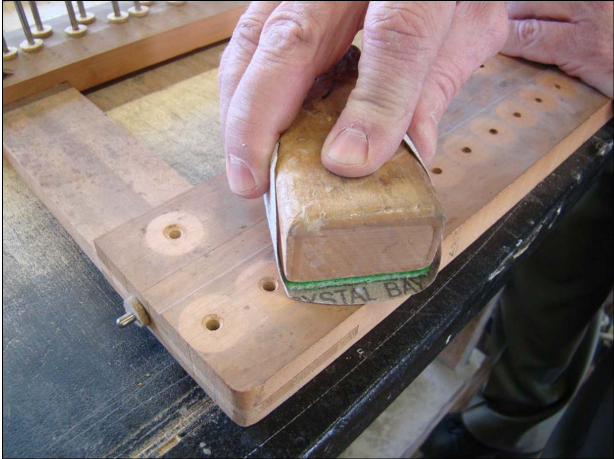
Figure 15 Sand front rail to clean and remove burrs
