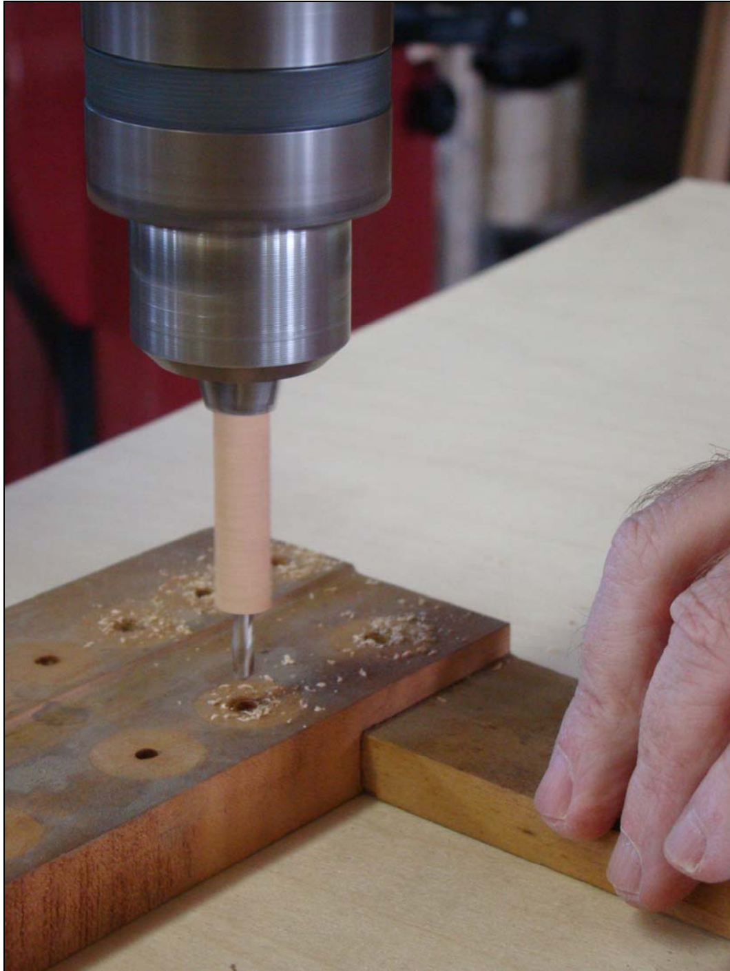
Figure 13 Drilling the front rail
