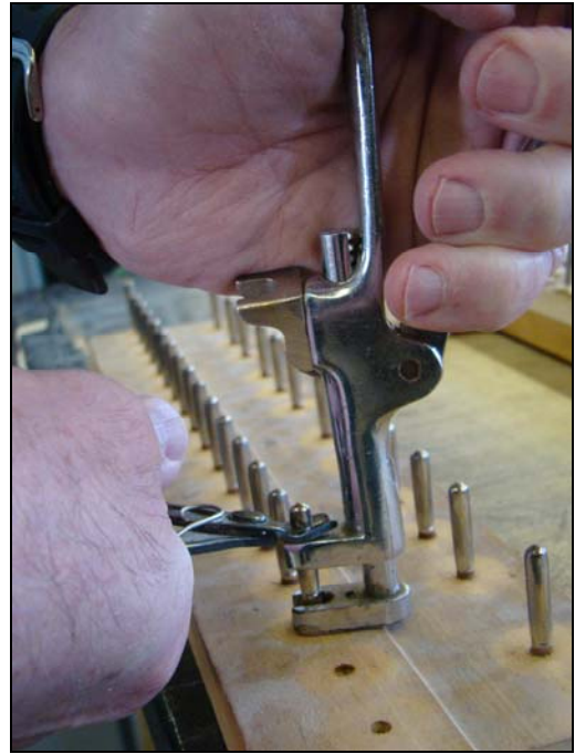
Figure 7 Removing front rail pins with side cutter and puller
