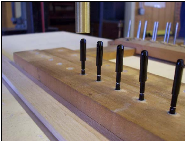
Figure 22 Drill press set up with Front Rail Pin Insertion Tool
