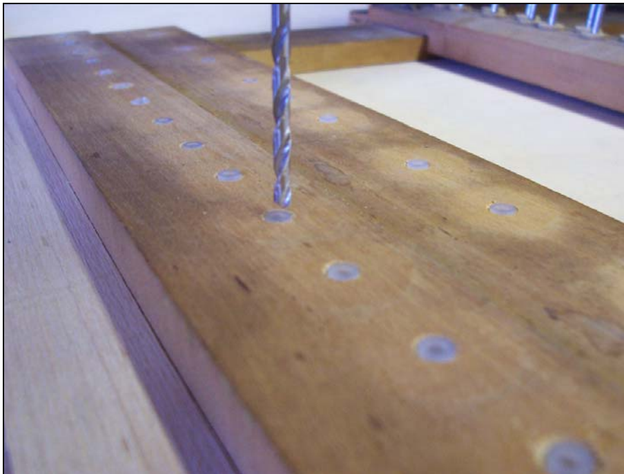
Figure 20 Drilling Nylon Bushings in the front rail
