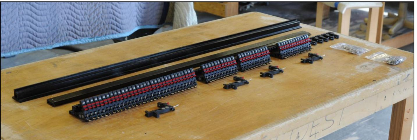
The kit you ordered includes an un-drilled Damper Flange Rail, an un-drilled Damper Sustain Tray, the correct quantity of underlevers with
