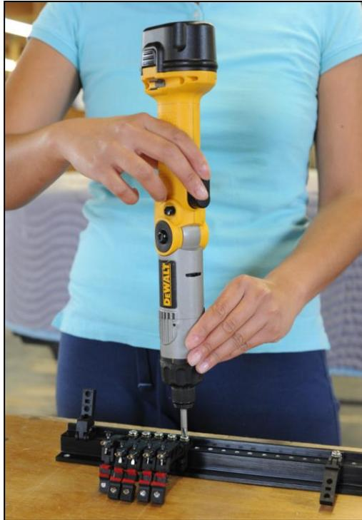
Assemble the underlevers to the flange rail in the correct order. Use a screwdriver to tighten with moderate tension the screws to fasten the underlevers to the rail.
