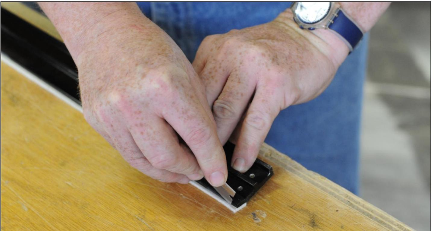
After the contact cloth is attached, it must be trimmed. Use a razor blade to trim the cloth to the damper tray.
