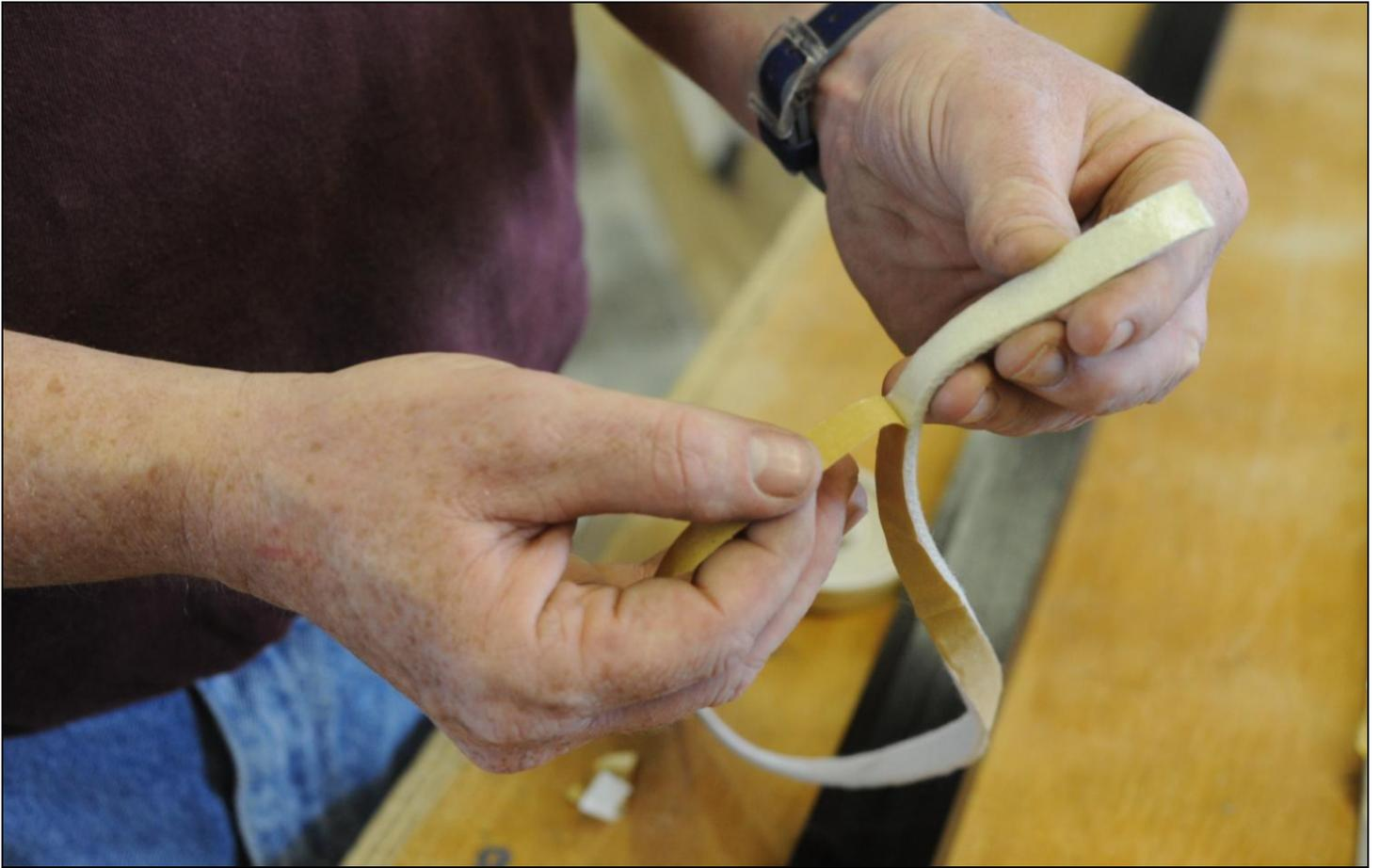
WNG uses self sticking contact cloth where the tray picks up the underlever. The first step is to peel back the backing paper.
