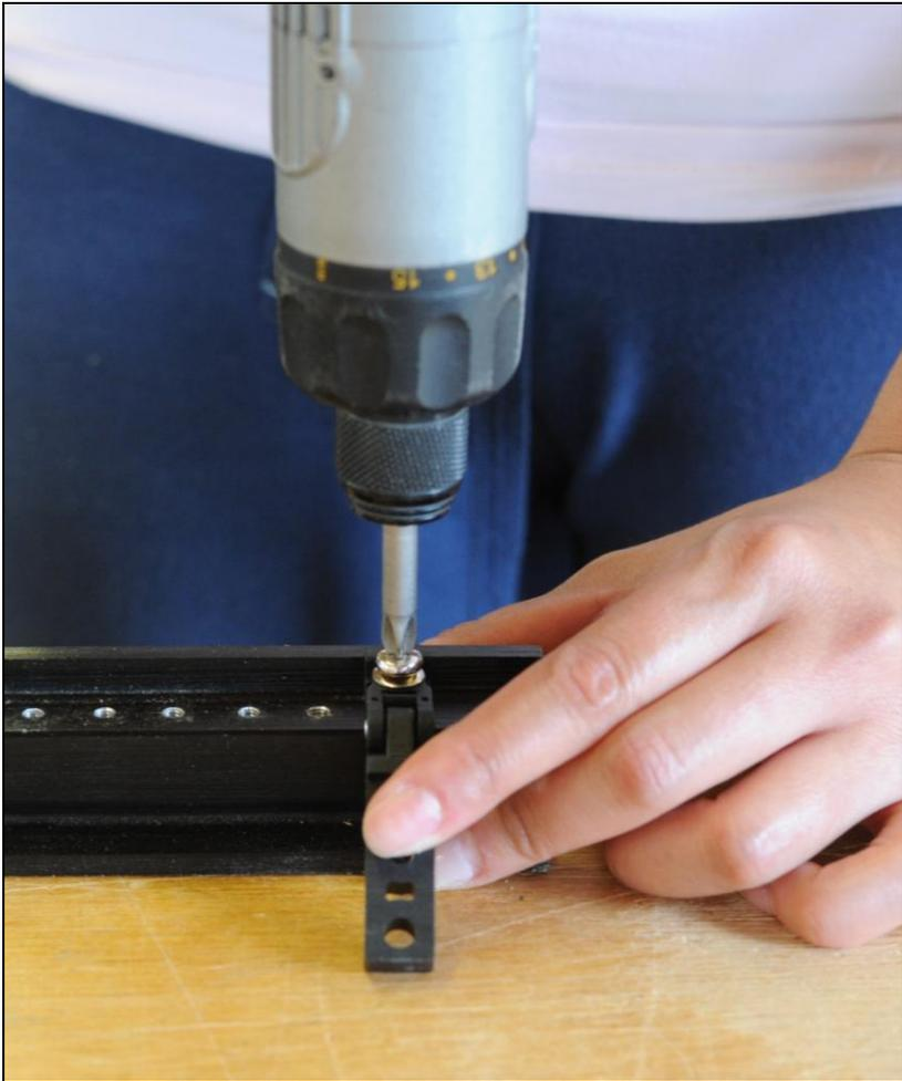
Assemble the tray flanges to the flange rail. Tray flanges use the same screws as the underlever flanges.
